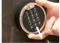
Now turn the keypad clockwise a few degrees until it comes to a stop. The columns of numbers should now be straight up and down. Your installation is complete. Before closing the safe door, and after installing a battery (as shown below), test the lock and keypad operation by following the operating instructions for your lock.
