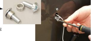
Then install the screws into the keypad mounting holes in the safe door. Note that the lock is already installed, and its cable is coming through the spindle hole.
