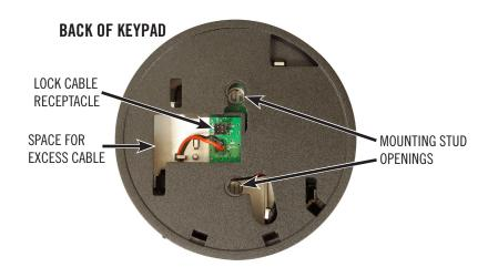
**Attaching Screws:** Use only the screws provided with the keypad. Mounting screws will be either 8-32 or M4, depending on the application. They must engage the mounting surface (safe door) by at least four full threads. Do not use thread sealing compounds as these may
