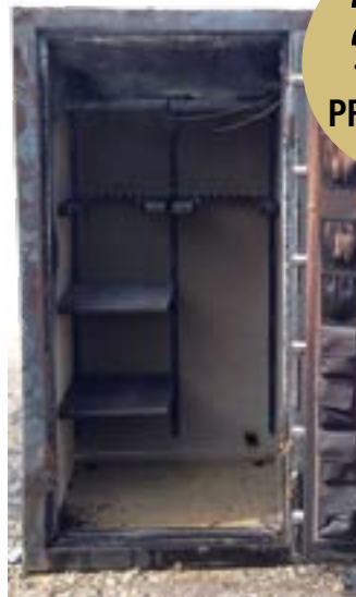
Browning ProSteel Safe with 1-7/8" thick insulation after 100 minutes at 1680° F.
