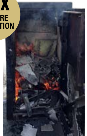
Leading U.S. built competitor safe with 1-7/8" thick insulation after 100 minutes at 1680° F.
