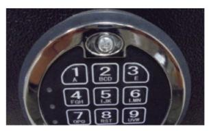
Carefully remove the keypad cover from the housing. Let the keypad cover hang with the wires still attached.
