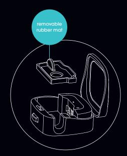
Yes, even Sanitizers need cleaning. To do so, remove and wash the silicone mat with water and then towel dry. For the interior and exterior case, all you'll need is a gentle wipe with a damp towel.
