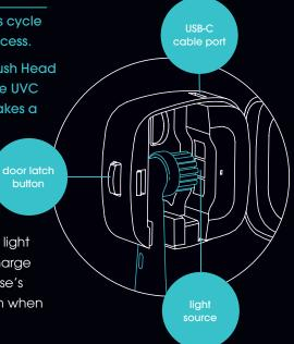
When you see the indicator light flashing red, it's time to recharge via the USB-C cable. The case's indicator light will turn green when
