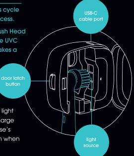
When you see the indicator light flashing red, it's time to recharge via the USB-C cable. The case's indicator light will turn green when fully charged.
