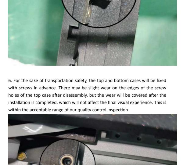
7. The ZOOM65 V3 taillight edition has a soft light strip inside the upper case. After disassembly and assembly, there is a gap between the upper and lower case, which will affect the soft light strip. Do not press and lock it immediately during the assembly
