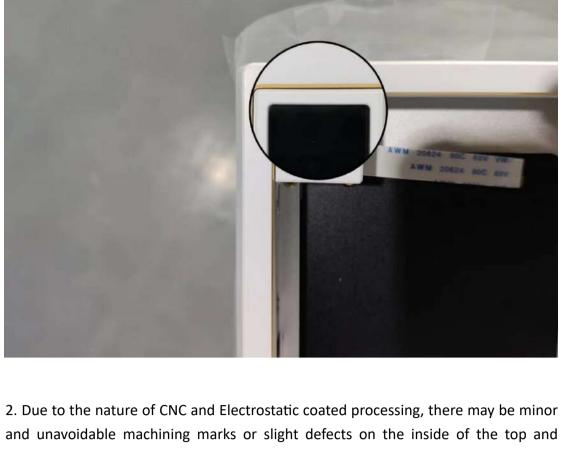
bottom case. However, once the keyboard is fully assembled, these marks do not
