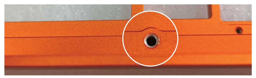
4. After the kit is assembled, there may be slight gaps depending on the individual's hands-on ability. Our quality control standard for gaps is ≤0.2mm. If the assembly gaps of the appearance parts exceed 0.2mm after assembly, please remove the screws and adjust. If the gap is still greater than 0.2mm after adjustment, please contact our customer service for a replacement or after-sales service.
