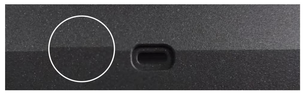
6. Because of the limitations of the PVD coating process on stainless steel, it is challenging to achieve a mirror surface completely free of hairline marks and pits. The visible distance of dust spots is 30cm; any dots on the surface smaller than 0.1mm and no more than 2 dots or scratches on the entire surface will be considered acceptable according to our quality control standards.
