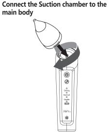
Insert the assembled suction chamber set into the suction port of the main body, rotate it clockwise to ensure it fits tight. Make sure it will NOT fall off in any angle.
