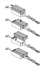
Figure 4.2.3 Lithium-ion Battery Replacement
