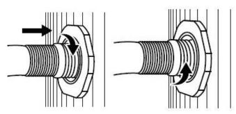
Turn both the hose and valve ¼ clockwise. Then insert ½ way to prepare draining. Once you have finished draining, turn the hose and valve ¼ counter-clockwise to remove.
