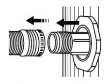
Remove the hose from valve and replace cap.
