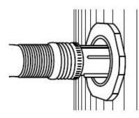
When cap has been removed, attach hose to extended valve.
