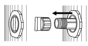
Locate closed valve. Pull closed valve backwards (fully extended) and remove cap. Place cap in safe place.
