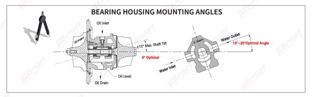
**C.** On internal WG units the WG must have the actuator realigned to suit any new position and preload reset.
