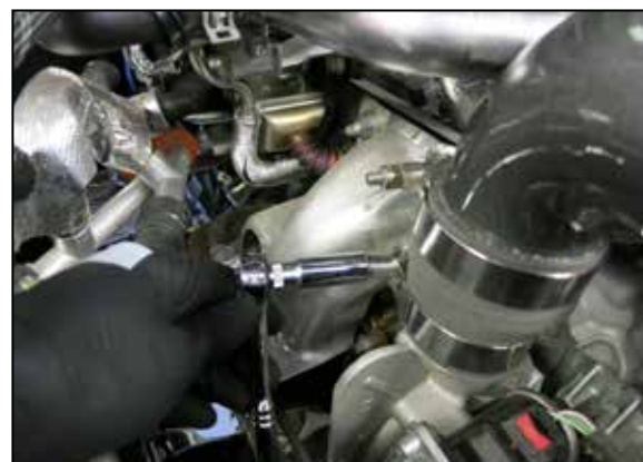
24. Remove the BOV from the factory charge tube and install it onto the K&N BOV manifold using the provided hardware.
