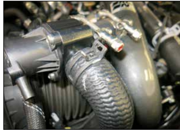
29. Install the BOV assembly onto the charge pipe and position so the outlet aligns with the BOV hose, Install the BOV hose onto the BOV and secure with the factory spring clamp. Then tighten the hose clamp to secure the valve assembly on to the charge pipe.
