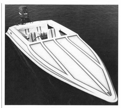
we could raise the engine and trim it out to a point where the boat chinewalked noticeably, but the condition didn't become a major concern until we passed 70 mph. At speeds in the mid to upper 60s, the Vegas was responsive, controllable and wellmannered.
