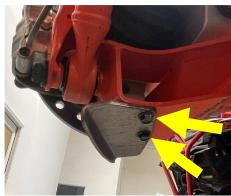
REMOVE THE MUD SCRAPER BY USING A 13MM SOCKET ON THESE TWO BOLTS
