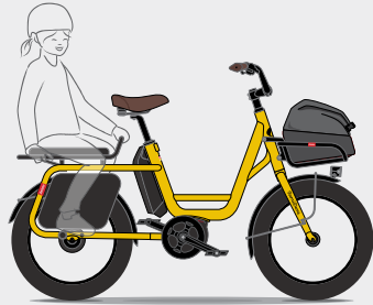
Carry a passenger (85lbs/40kg max) with Passenger Kit and Jump Seat Rear Rack.
