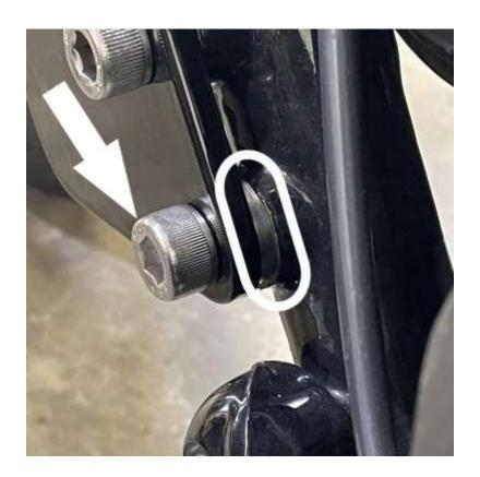
**Step 5 :** Once the bars is adjusted, tighten the bottom bolts at first, the top bolt on the throtle side in second, and finish with the locknut (Hardware number 5) on the clutch side.
