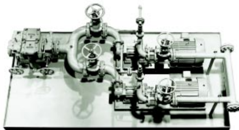
Main and standby 3D-218 fuel pumps on common skid with inlet strainer, discharge relief valves and block valves.
