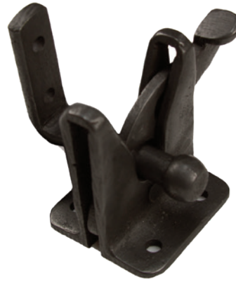
Standard Gate Latch - Offset 50-205 Dimensions: 2" L x 2" W x 1-3/4" H Catch: Offset Screw: 1" Round | #10 Stainless
