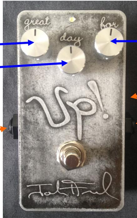
The pedal has an internal switch for a buffered bypass. You can use the buffer to help boost your signal through a long line of true bypass pedals, which will sap your tone a little. The pedal comes with the switch set to true bypass.
