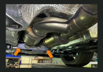
**Step 8**Unbolt both bolts in order to remove the downpipe hanger mount.
