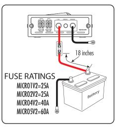
Securely mount the amplifier to the vehicle or amp rack. Be careful not to mount the amplifier on cardboard or plastic panels. Doing so may enable the screws to pull out from the panel due to road vibration or sudden vehicle stops.
