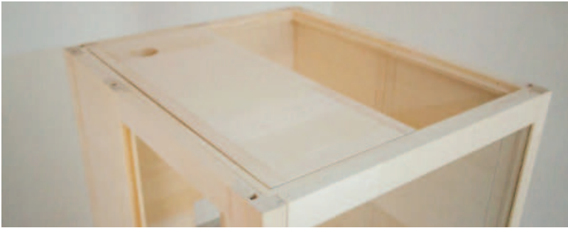
Fig. 14: Inserting front ceiling element
