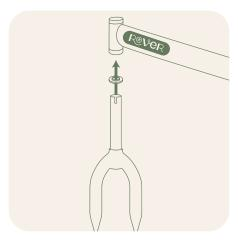
Slide flat washer on the front fork. Then, insert to the front of the main frame.
