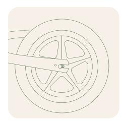
7 Slot the wheel axis into both ends of the fork.
