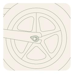
8 Position the hooked washer on the wheel axis.
