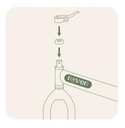
3 Slide rounded washer and place clamp D on top of the front fork.
