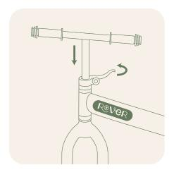
Insert handle bar. Adjust to a suitable height and tighten the clamp.
