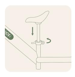
6 Insert saddle post. Adjust to a suitable height and tighten the clamp.
