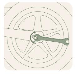
Oap with nut. Tighten nut with a spanner tool. Repeat for all sides.
