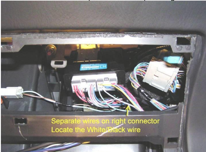
Photo 3 - Convertible Top Module and Speed Signal Wire
