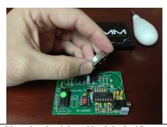
6. Place the circuit board back in the iComm top casing (label side). Then re-attach the back case. Re-insert the screw to the back case.
