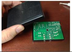
4. Gently pull the battery straight upward from the circuit board until it releases.
