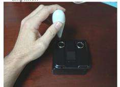
2. Face the speaker down and remove the back of the amplifier casing.
