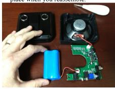
4. Pull out the battery and unplug the battery cable from the circuit board. Plug in the new battery to the circuit board.
