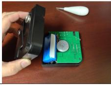
3. Note the location of the circuit board and battery so that you can return to the proper place when you reassemble.
