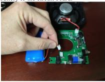
5. Place the circuit board and battery back into it's original position. Put the back of the amplifier case back on the amplifier.
