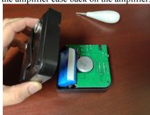
6. Put the 4 screws back into the case back of the amplifier.
