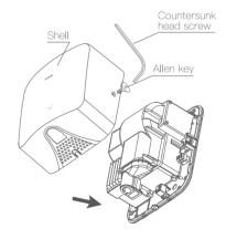
4. Reinstall the shell and screw on the 2 countersunk head screws on the side.
