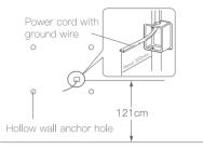
1. When installing the hand dryer without a junction box, you need to install a standard socket corresponding to the hand dryer on the upper right side of the hand dryer, with a distance of 20–50 cm. If you need to connect the power cord directly, please insert a coverless junction box at the installation location. (If the junction box is not used, the power cord will be squeezed out of the body and affect the installation.)
