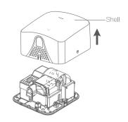
2.Remove the 2 countersunk head screws on both sides of the hand dryer, hold the shell up with both hands and remove it with force. The shell must be kept in a safe place to avoid scratches.
