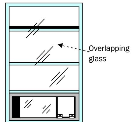
**Step 6:** Unroll the strips of fuzzy gray pile weather-stripping and feed them into the channels running along the window panel. These channels will be on the sides of the panel that the window will close against. Therefore, if you have a vertically opening window, the channels will be on the top and bottom of the window insert. If you have a horizontally opening window, the channels will be on the two sides of the window insert.
