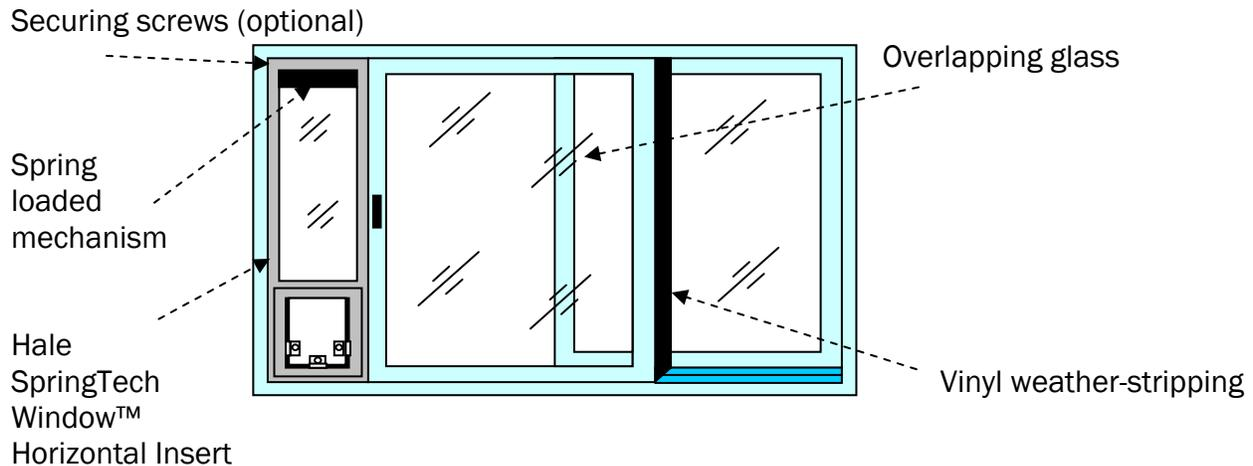
**Step 14:** If you so desire, you can put a screw or two through the window frame to prevent the window from being opened. **Be very careful that you don't drill into glass!** If you hit the window pane with either the tip of the drill bit or a screw, it will shatter. The glass in the pet door comes all the way to the edge of the frame, so don't try to drill into the pet door frame at all.
