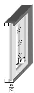
ADJUSTMENT AREA ON THE OMNI MODEL BUT PLEASE MEASURE CAREFULLY. MEASURE DOWN INSIDE THE BOTTOM TRACK AND FLUSH WITH THE TOP TRACK. DO NOT MEASURE INSIDE BOTH TRACKS OR THE WINDOW WILL BE TOO TALL. DO NOT MEASURE FLUSH ON BOTH ENDS OR THE WINDOW WILL BE TOO SHORT. SEE GRAPHIC BELOW FOR DETAILS.
