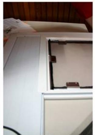
When installing the spline in the corner of the pet door unit, it may be necessary to cut a small diagonal slit up into the screen material in order to relieve the tension on the screen
