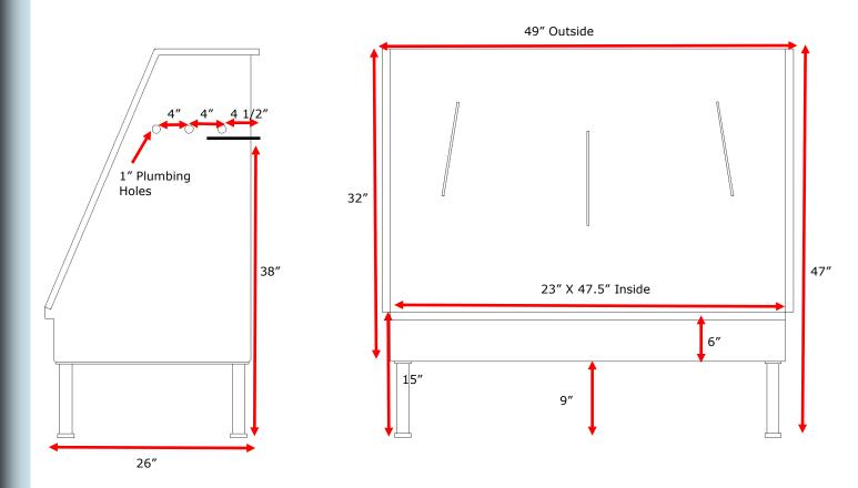
Faucet holes and drain are available on the left, right or center. The drain hole is  $3 \, 1/2''$  in diameter and is centered from front to back in the tub, which puts the center of the hole at 12'' from the front and 12'' from the back and  $7 \, 1/2''$  from the side of the tub. The three faucet holes are 4'' on center. The holes are 1'' in diameter and are up 29'' from the bottom of the tub basin or approximately 38'' from the floor.
