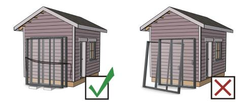
Handle and stack frames carefully on site. Stand them upright on their sills (bottom of the window as installed), raised off the ground on pieces of timber or bricks. Stand them against a flat, vertical surface such as a shed and tie firmly in position.
