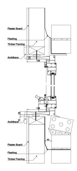
french door open inward & open outward Plaster Board Flashing . . . . Timber Framing Architrave Flooring Architrave Architrave С  $\bigcirc$ B−/B Plaster Board  $\bigcirc$ Plaster Board Flooring Slab A Flashing Flashing Flashing  $\bigcirc$  $\bigcirc$  $\bigcirc$  $\bigcirc$ 0  $\bigcirc$  $\bigcirc$  $\bigcirc$ Ð  $\bigcirc$  $\bigcirc$  $\bigcirc$  $\bigcirc$  $\bigcirc$  $\bigcirc$  $\bigcirc$   $\bigcirc$  $\bigcirc$  $\bigcirc$  $\bigcirc$  $\bigcirc$  $\bigcirc$  $\bigcirc$ A-A
