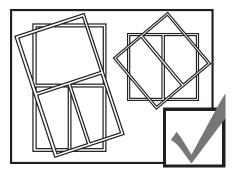
Do not lean windows against a tree or post as they are subject to permanent damage until installed into the building envelope. If the site is bare, lay frames flat on top of each other with weight evenly distributed to avoid buckling and distortion.
