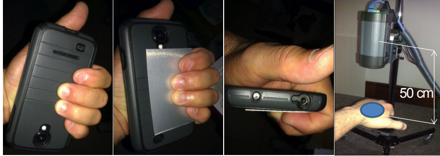
Figure 2: Hand test with a Galaxy S4 and a Bodywell card (Picture not to scale, phone cover removed during tests).
