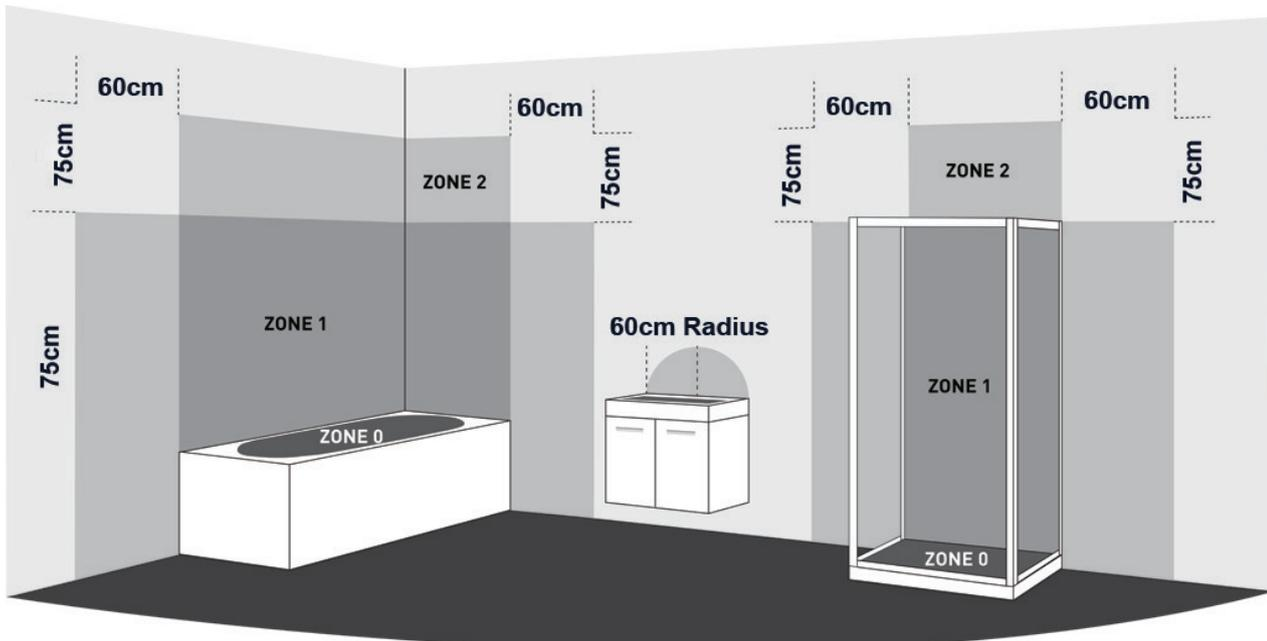
This product is IP44 rated and is suitable for installation within zone 2 above, and complies with the following safety standards: BS EN 60598-1: 2008+A11: 2009, EN60598-2-1: 1989
