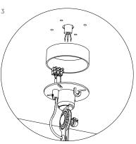
Install 3. Terminal block to install directly on a junction box with optional ceiling.
