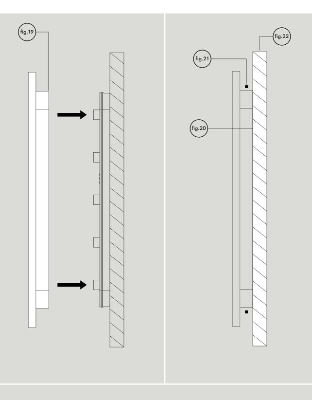
Install the cover assembly (fig.19). Ensure edge of cover (fig.20) is flush against the surface (fig.22). To achieve this gently push the cover until the edge is touching the surface (fig.22). Whilst holding the cover against the surface secure with 2X set screws (fig.21).
