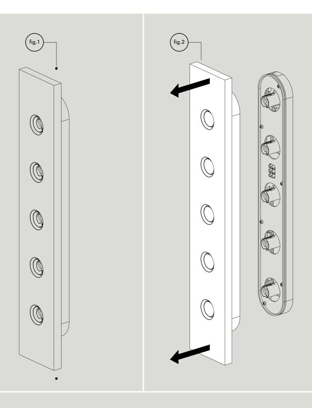
Loosen both upper and lower set-screws (fig.1). Gently remove cover assembly (fig.2), taking great care not to damage the lamp holders.
