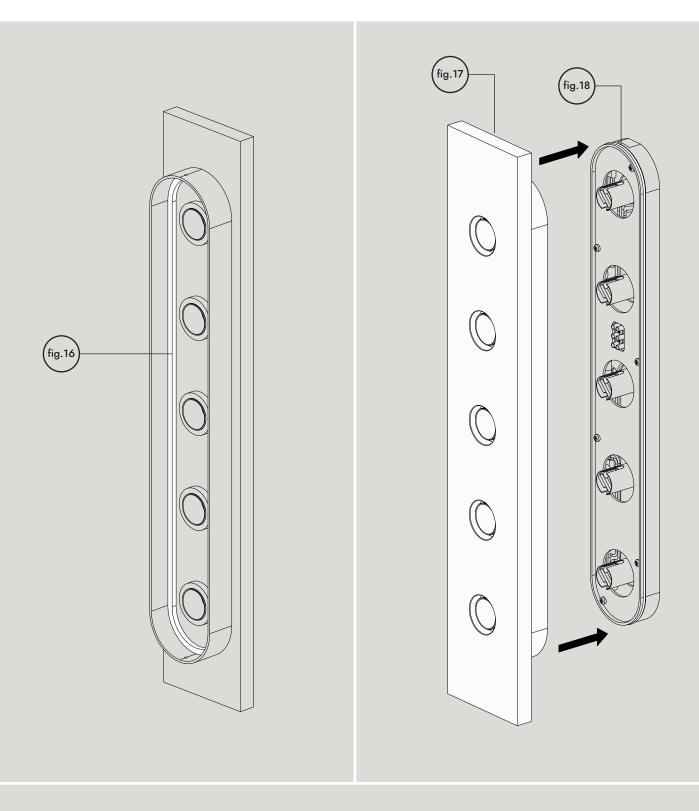
Gently install cover assembly (fig.17). Line up all five holes and mate cover assembly with main body. Take great care not to damage the lamp holders. You will feel slight resistance due to the groove gasket (fig.18), this is normal. Inner gasket (fig.16) will compress against outer edge of the main body.
