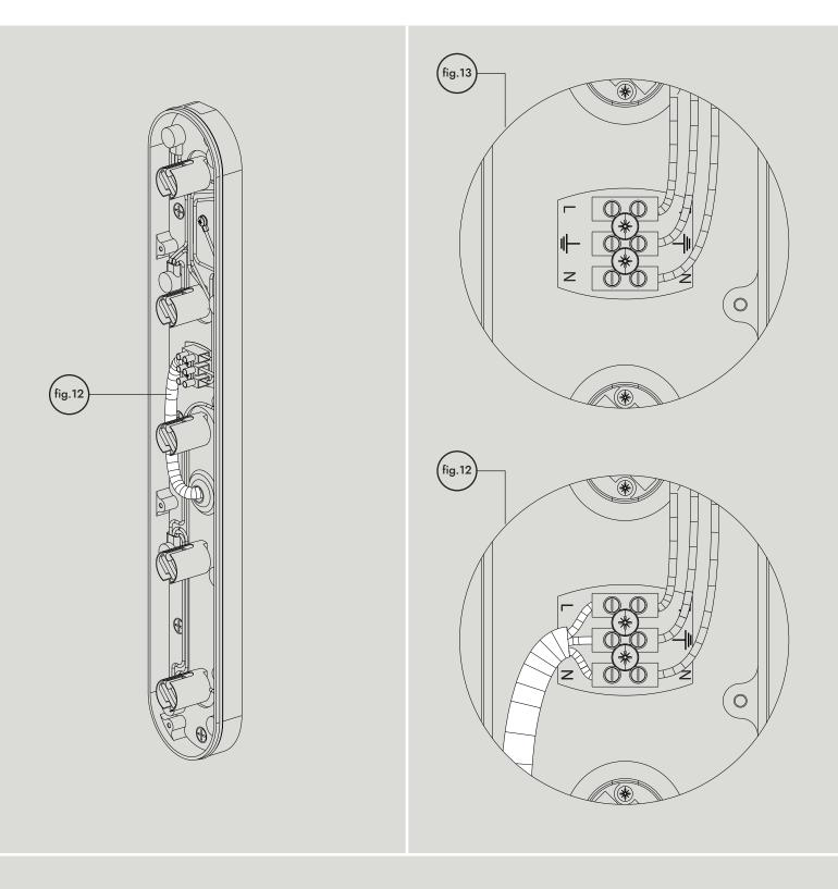
Connect the mains cable to the terminal block (fig.12). L = Brown, N = Blue Earth = Green & Yellow (fig.13).
