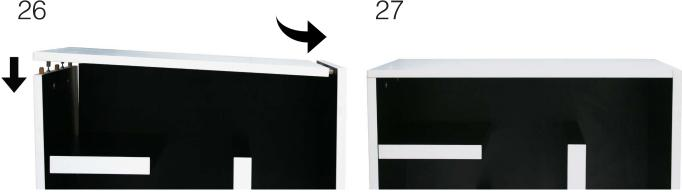
Before placing the caps make sure to tighten firmly all the minifix hardware
