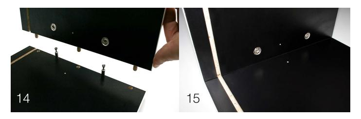
Tighten the minifix hardware clockwise
