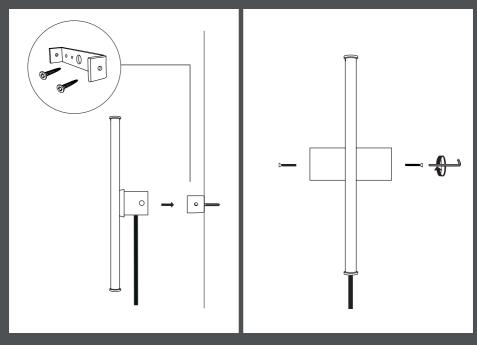
Detach the mounting plate from the wall lamp and mount it to the wall. Make sure to use appropiate screws and rawlplugs/anchors. Mount the wall lamp to the plate on the wall using the plated screws. Turn the screws clockwise for fastening.
