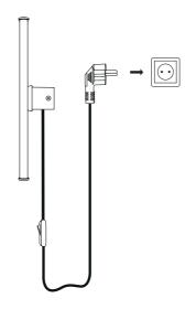
Plug the socket into a power outlet. If there is a built in lamp socket in the wall, the lamp can also be mounted directly to the wall without the cable.
