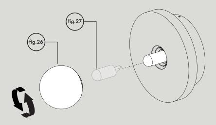
To replace LED capsule. Gently unscrew glass shade (fig.26). Hold the LED capsule (fig.27) firmly and pull in a parallel motion from the lamp holder. Do not twist as this could damage the lamp holder. To fit LED, firmly push LED into lamp holder. Ensure secure fit.
