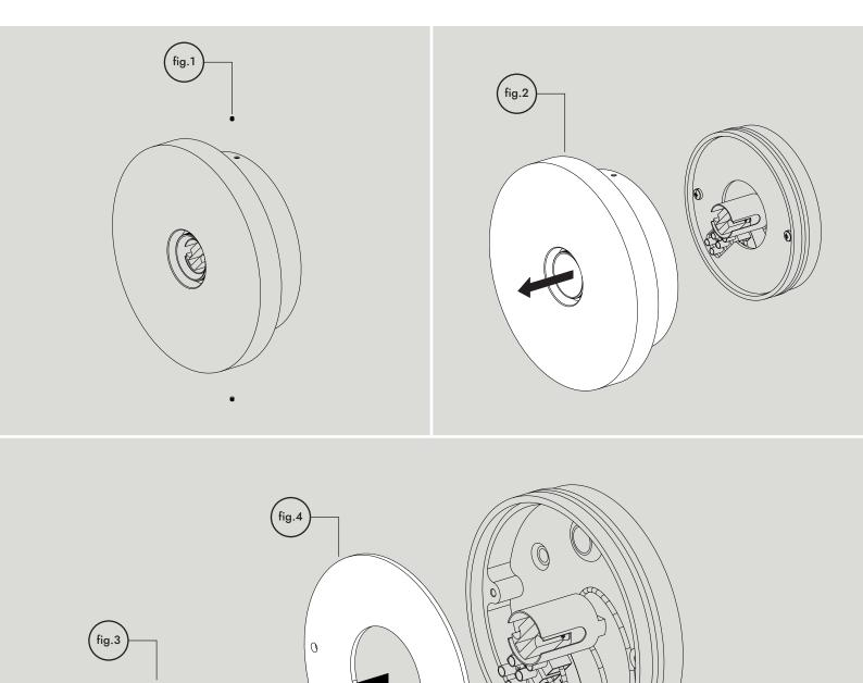
Loosen both upper and lower set-screws (fig.1). Gently remove cover assembly (fig.2), taking great care not to damage the lamp holders. Unscrew 2X cover screws (fig.3) and remove cable cover (fig.4).
