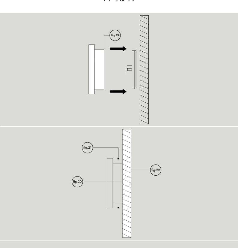
Install the cover assembly (fig.19). Ensure edge of cover (fig.20) is flush against the surface (fig.22). To achieve this gently push the cover until the edge is touching the surface (fig.22). Whilst holding the cover against the surface secure with 2X set screws (fig.21).
