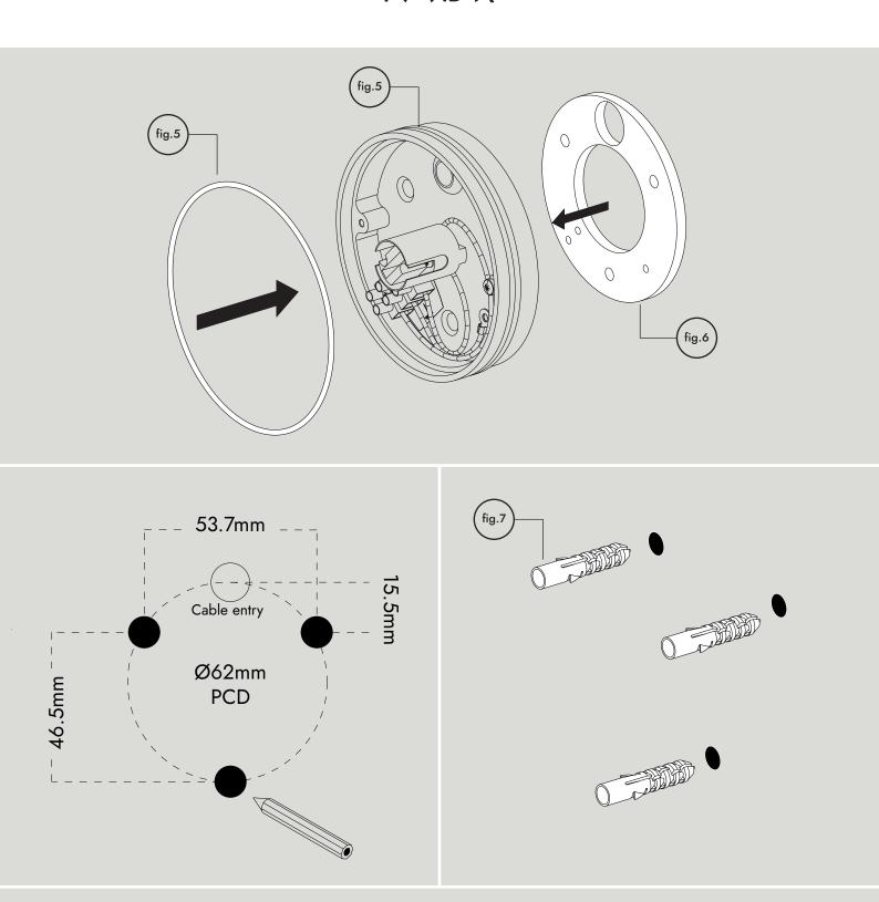
Fit gasket (fig.5) into groove on the body. Gently stretch gasket until fit is achieved. Ensure wall gasket (fig.6) is positioned within its allocated space at the back of the product. Ensure wall is flat and free from imperfections. Mark out mounting holes. Pay attention to position of cable entry to ensure correct final positioning of product. Drill holes for appropriate wall plug fixings, suitable for the fabric of the wall and fit wall plugs (fig.7) not supplied.
