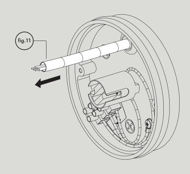
Mains cable from surface (fig.11) must be in line with cable entry on the body (fig.10). Offer cable from surface through the body. Fix body (fig.9) to surface using 3X screws supplied (fig.8). Ensure wall gasket is fully compressed on surface.
