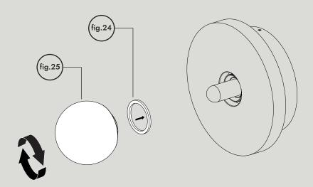
Install 1X G9 LED capsule Max 4W (fig.23) not supplied. Ensure capsule is firmly pushed in. Before screwing on glass shade (fig.25), ensure that 1X glass gasket (fig.24) is located in its place. Please take great care when handling the glass shade. Screw glass shade gently so its firmly secured. Do not over screw as this can cause the glass to break.
