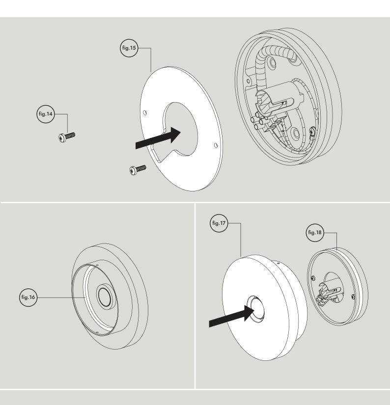
Fit cable cover (fig.15) with 2X screws (fig.14). Ensure that no cables are trapped or loose. Gently install cover assembly (fig.17). Line up hole and meet cover assembly with main body. Take great care not to damage the lamp holder. You will feel slight resistance due to the groove gasket (fig.18), this is normal. Inner gasket (fig.16) will compress against outer edge of the main body.
