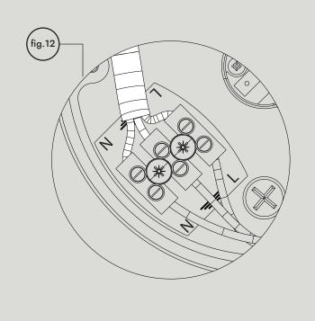
Connect the mains cable to the terminal block (fig.12). L = Brown, N = Blue Earth = Green & Yellow (fig.13).
