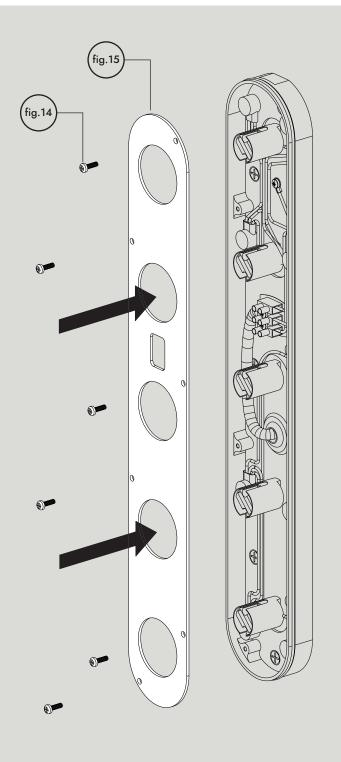
Fit cable cover (fig.15) with 6X screws (fig.14). Ensure that no cables are trapped or loose.
