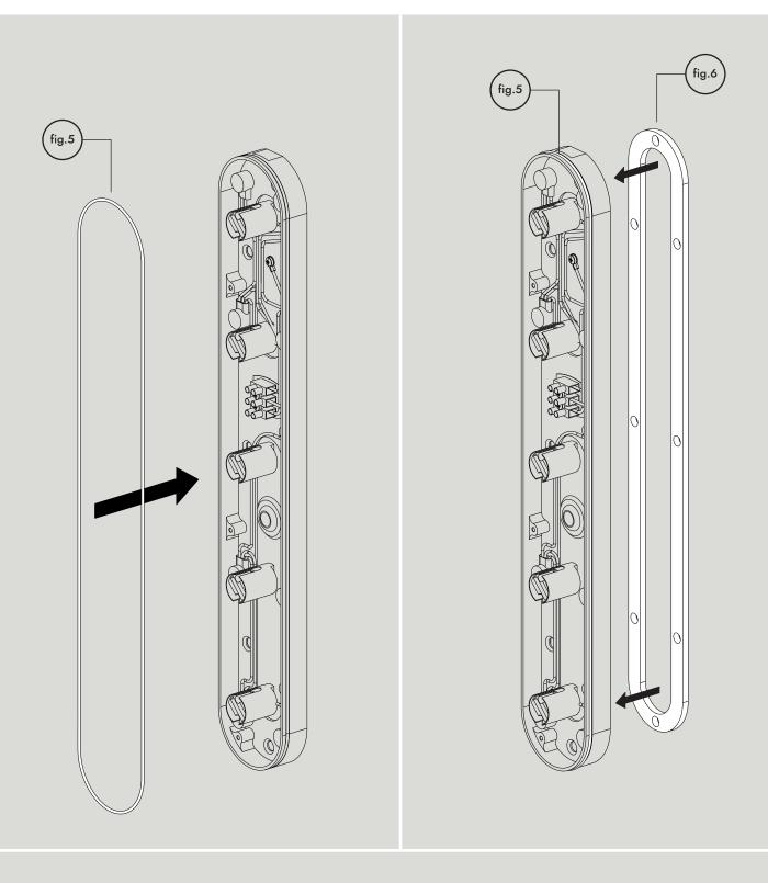
Fit gasket (fig.5) into groove on the body. Gently stretch gasket until fit is achieved. Ensure wall gasket (fig.6) is positioned within its allocated space at the back of the product.
