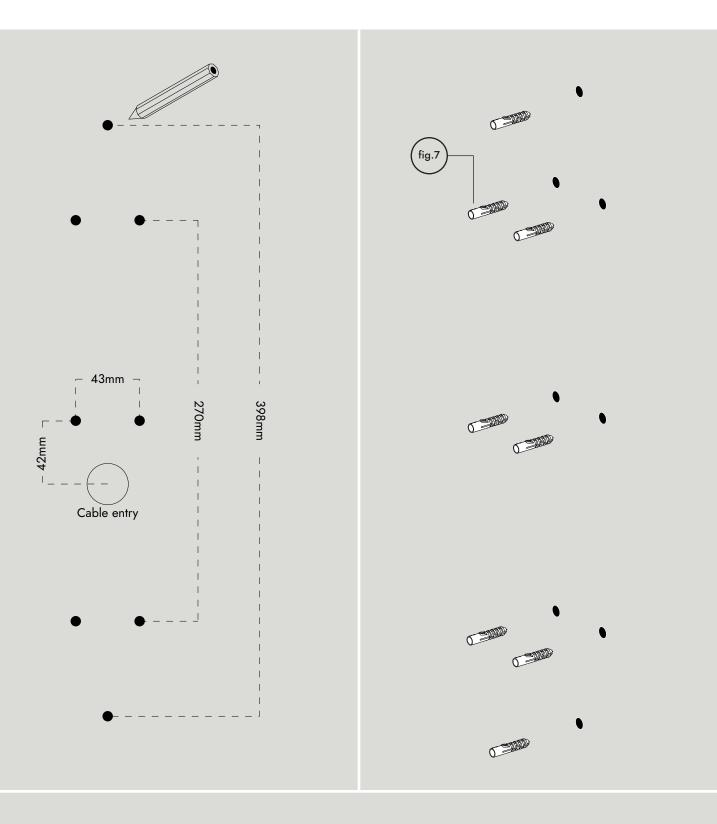
Ensure wall is flat and free from imperfections. Mark out mounting holes. Pay attention to position of cable entry to ensure correct final positioning of product. Drill holes for appropriate wall plug fixings, suitable for the fabric of the wall and fit wall plugs (fig.7) not supplied.
