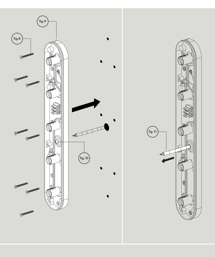
Mains cable from surface (fig.11) must be in line with cable entry on the body (fig.10). Offer cable from surface through the body. Fix body (fig.9) to surface using 6X screws supplied (fig.8). Ensure wall gasket is fully compressed on surface.
