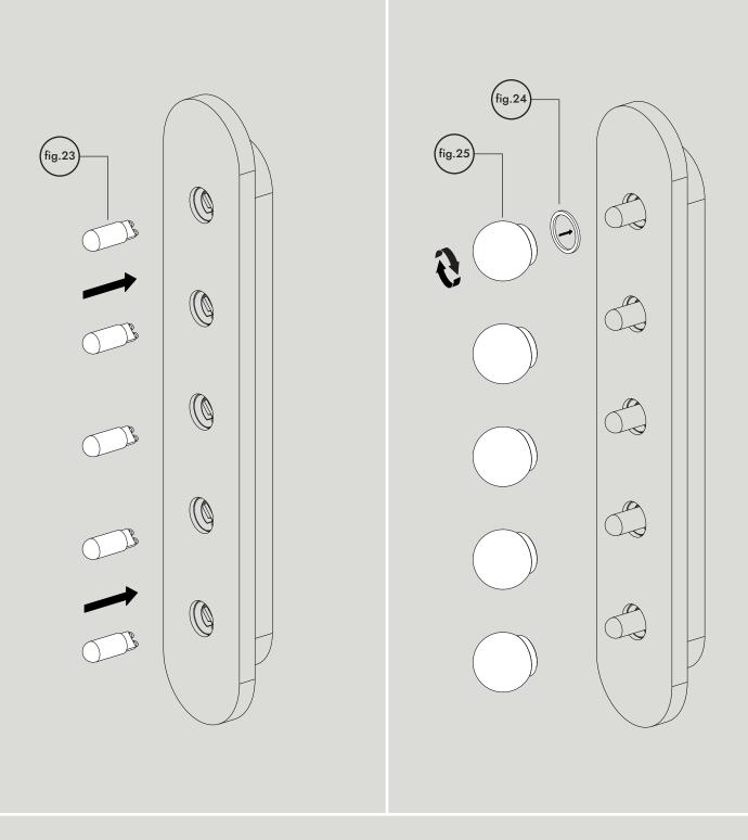
Install 5X G9 LED capsule Max 4W (fig.23) not supplied. Ensure capsule is firmly pushed in. Before screwing on glass shade (fig.25), ensure that 1X glass gasket (fig.24) is located in its place. Please take great care when handling the glass shade. Screw glass shade gently so its firmly secured. Do not over screw as this can cause the glass to break.
