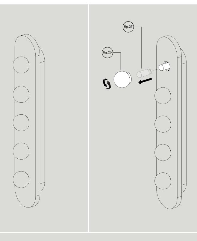
To replace LED capsule. Gently unscrew glass shade (fig.26). Hold the LED capsule (fig.27) firmly and pull in a parallel motion from the lamp holder. Do not twist as this could damage the lamp holder. To fit LED, firmly push LED into lamp holder. Ensure secure fit.
