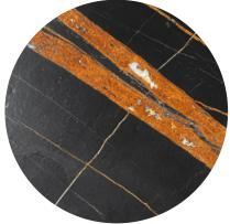
**Brushing** finish is obtained using tools equipped with abrasive brushes; this technique confers an orange-peel appearance, with a slightly wavy texture evocative of silk.
