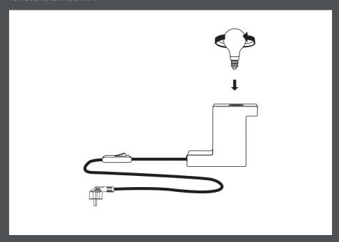
1. Place a recommended light bulb in the E14 socket.
