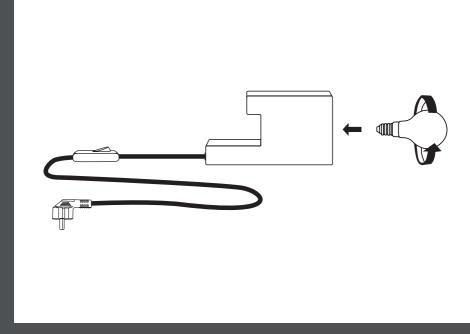
Place a recommended light bulb in the E14 socket.
