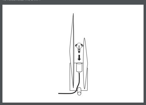
1. Place a recommended light bulb in the E14 socket. Light bulb is not included.
