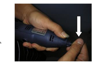
Hold D-160 drive open the collar and press the black button to lock it and unscrew the collar
