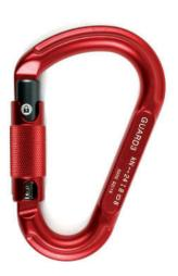
Type: H/B Length: 120 mm 76 mm Width: 22 mm Opening: Weight: 86 q Major axis 24 kN 8 kN Minor axis Open 8 kN Material: Light alloy
