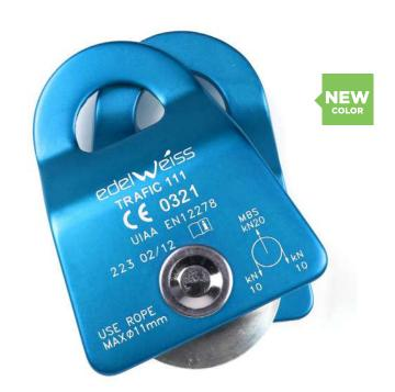
Height: 72mm Width: 58mm Sheave: 27,5mm 1 rope max.: 11mm Weight: 120 g
