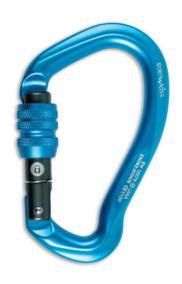
Type: H/B Length: 105 mm Width: 66 mm 20 mm Opening: Weight: 66 g Major axis: 28 kN Minor axis: 8 kN 8 kN Open: Material: Light alloy
