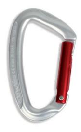
В Type: Length: 96 mm Width: 59 mm Weight: 44 g Major axis: 24 kN Minor axis: 8 kN Open: 7 kN Material: Light alloy CE - EN 12275 - UIAA Norm: Code: MTOPD
