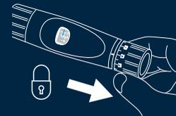
When not in use, adjust the wrench to its lowest reading, and store it in the provided case.
