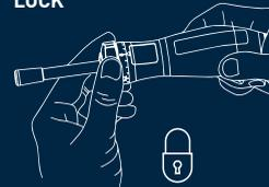
When not in use, adjust the wrench to its lowest reading, and store it in the provided case.
