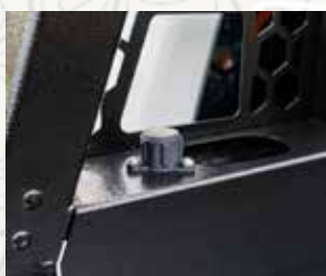
HEADBOARD FILL POINT FOR WATER TANK
