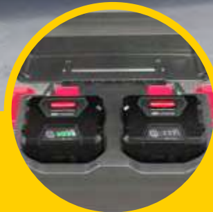
Dual onboard battery compartment provides back-up power storage without having to plug in the entire truck.
